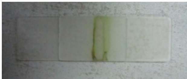
Figure 12. The welding of TGMPP and PA66.
