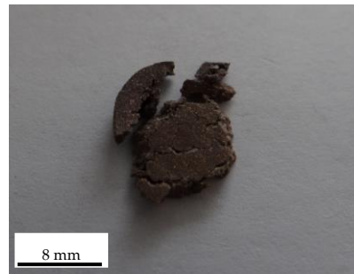
Figure 4. Failed PTFE/Cu sample.
