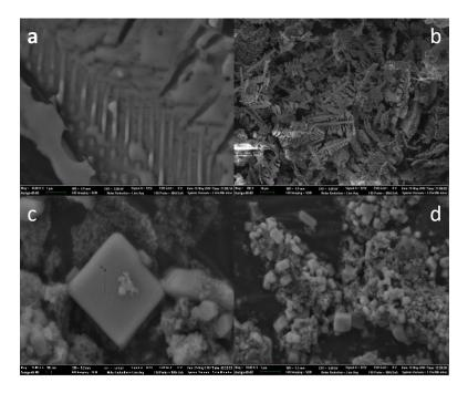
Figure 6. SEM images of calcium phosphate crystals (a,b), crystals with MBFA (c,d).
