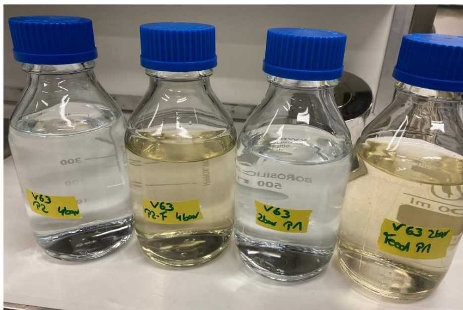
Figure 7. Photo of permeate and feed in an experiment with treated wastewater. From left to right: permeate at TMP = 4 bar, feed of the same experiment, permeate at TMP = 2 bar, and feed of the same experiment (Source: Oeltze).
