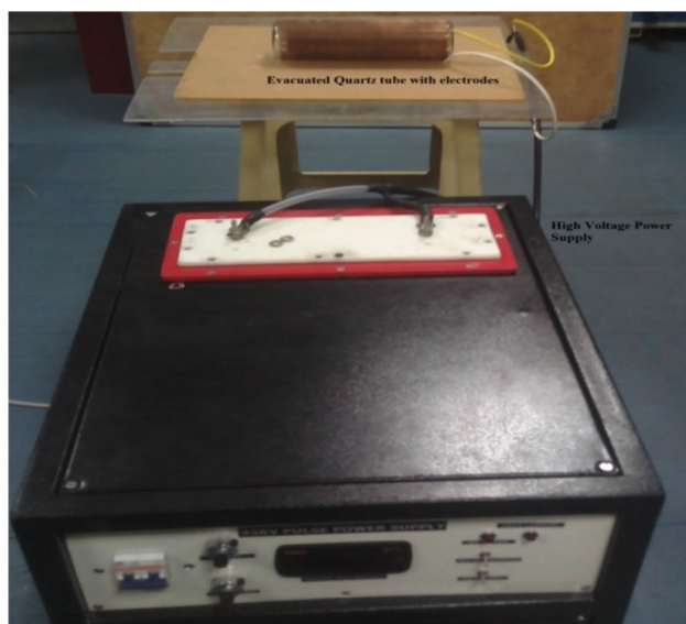
Fig. 4 DBD quartz tube with power supply
