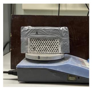
Figure 6. Hot plate setup. Labels: (A) insulation, (B) hot plate, (C) specimen.
