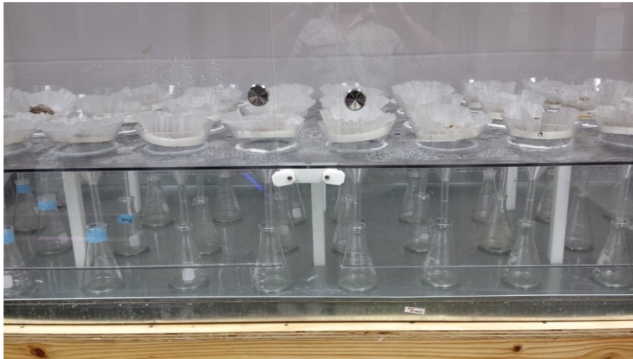
Figure 7: Samples are placed onto coffee filters on the sample support rings. Funnel necks insert slightly into the 250-ml-flasks.
