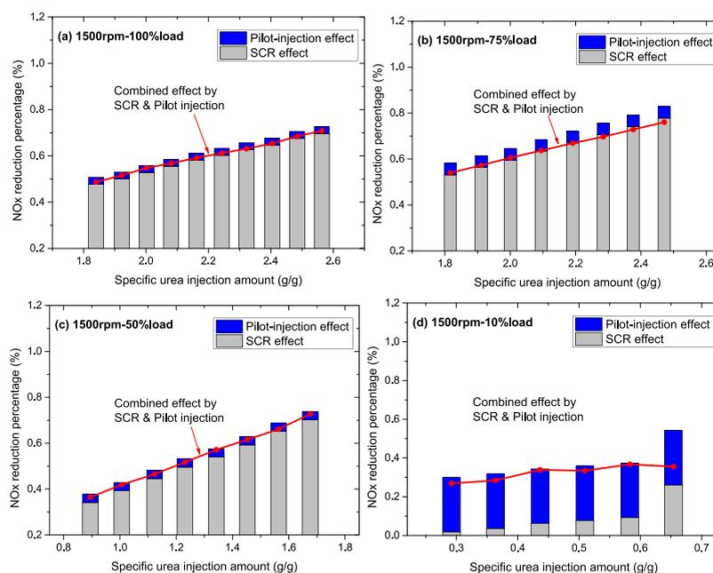
**Figure 8.** NOx reduction percentage by SCR and pilot injection and SCR + optical pilot-injection strategy for 1500 rpm engine speed conditions.
