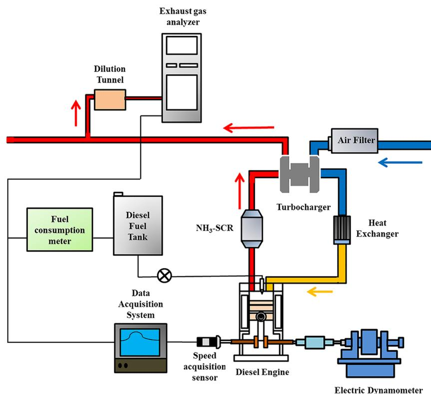
**Figure 9.** Schematic diagram of the engine test setup.
