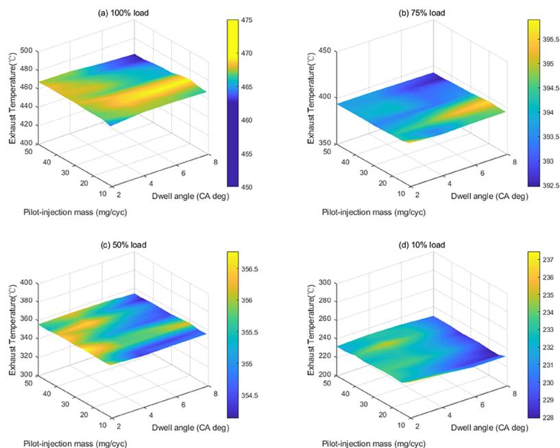
**Figure 5.** exhT for different interval angles and injected fuel masses of pilot injection at (a) 100% load, (b) 75% load, (c) 50% load, and (d) 10% load at a rated power speed of 2200 rpm.
