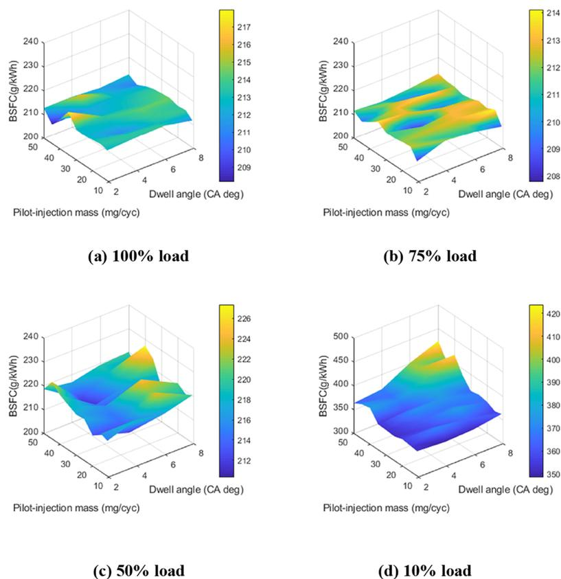
**Figure 4.** BSFC for different interval angles and injected fuel masses of pilot injection at (a) 100% load, (b) 75% load, (c) 50% load, and (d) 10% load at a maximum torque speed of 1500 rpm.
