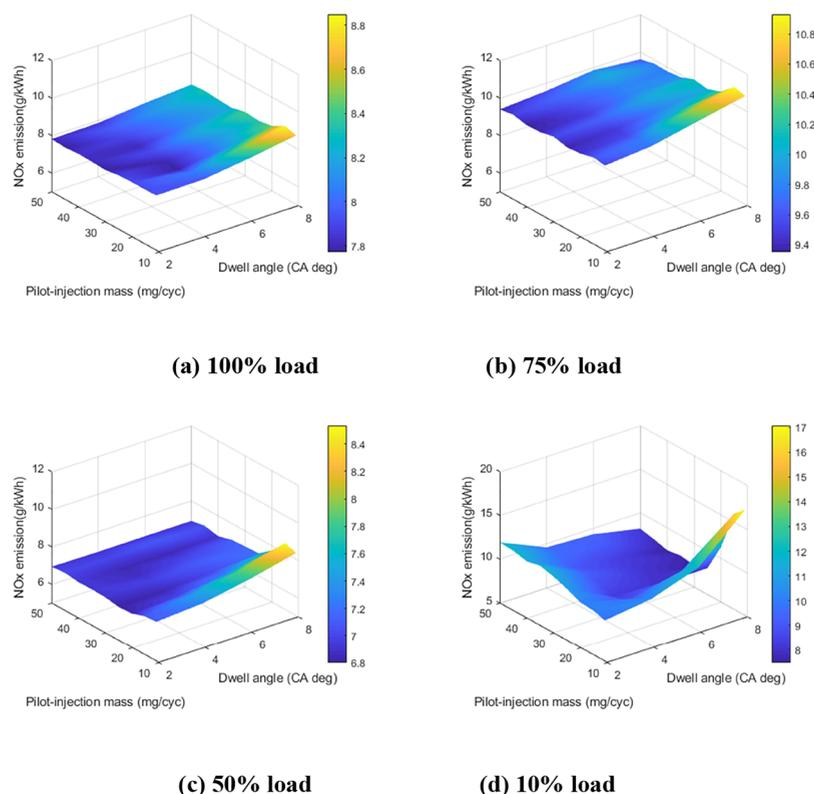
**Figure 2.** NO<sub>x</sub> emission for different interval angles and injected fuel masses of pilot injection at (a) 100% load, (b) 75% load, (c) 50% load, and (d) 10% load at a rated power speed of 2200 rpm.
