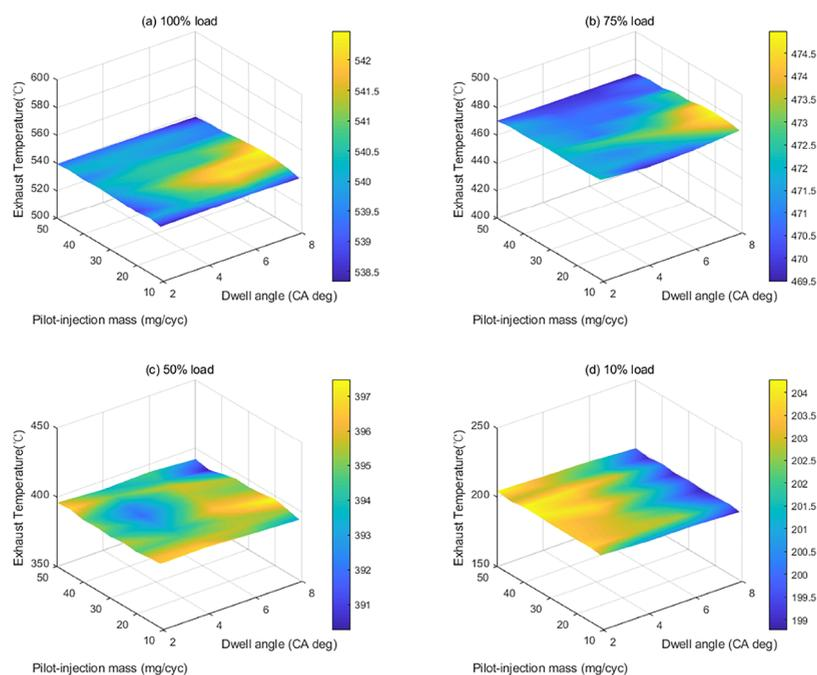
**Figure 6.** exhT for different interval angles and injected fuel masses of pilot injection at (a) 100% load, (b) 75% load, (c) 50% load, and (d) 10% load at a maximum torque speed of 1500 rpm.
