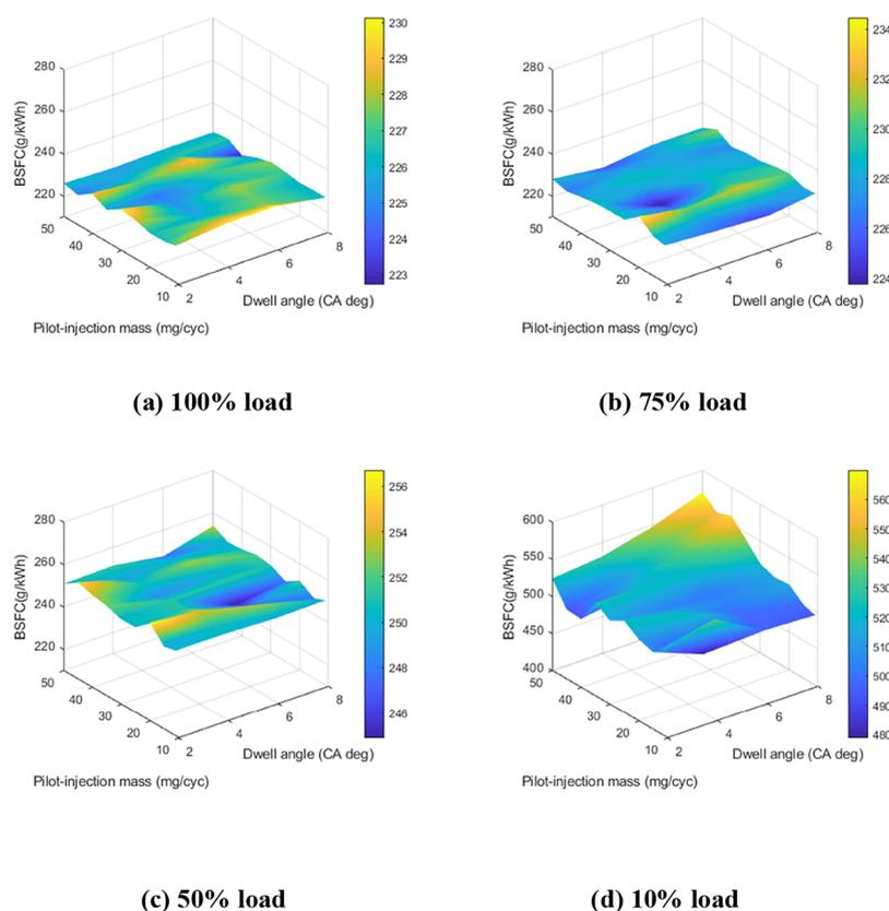
**Figure 3.** BSFC for different interval angles and injected fuel masses of pilot injection at (a) 100% load, (b) 75% load, (c) 50% load, and (d) 10% load at a rated power speed of 2200 rpm.
