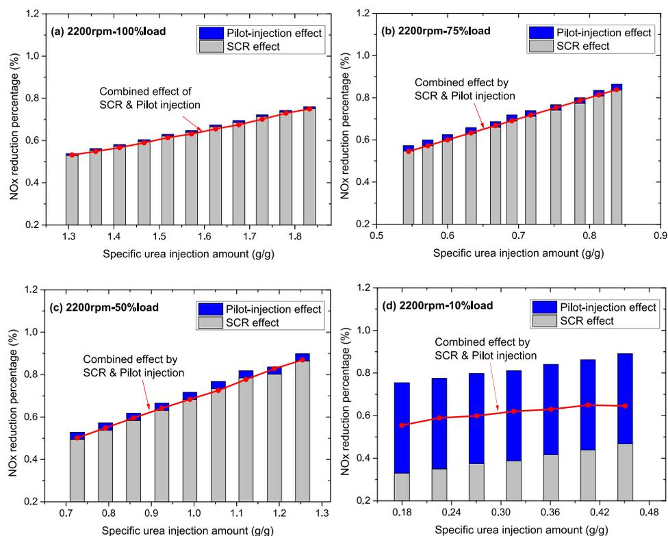
**Figure 7.** NO<sub>x</sub> reduction percentage by SCR and pilot injection and SCR + optical pilot-injection strategy for 2200 rpm engine speed conditions.
