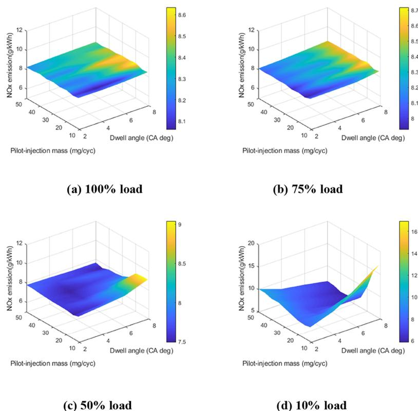
**Figure 1.** NO<sub>x</sub> emission for different interval angles and injected fuel masses of pilot injection at (a) 100% load, (b) 75% load, (c) 50% load, and (d) 10% load at a maximum torque speed of 1500 rpm.
