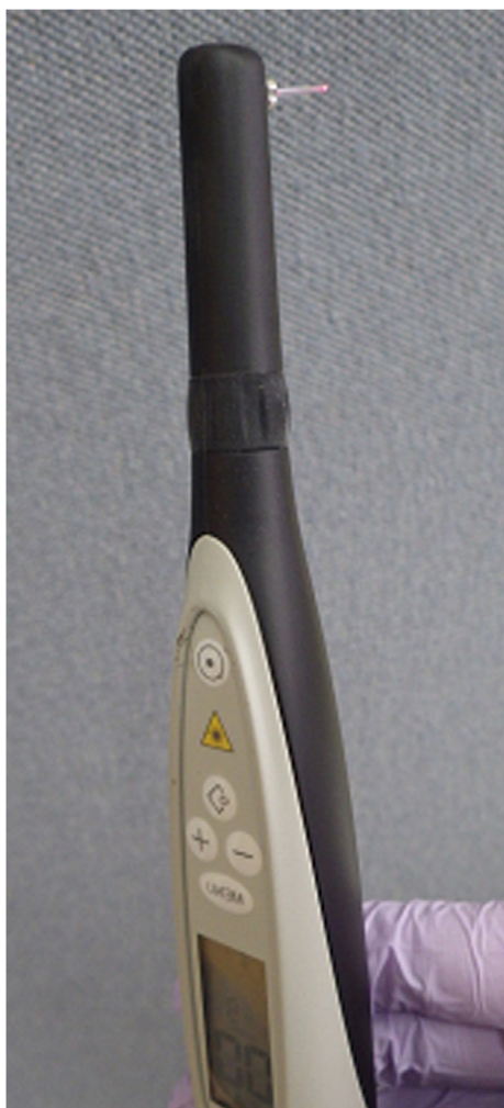
Fig. 1 DIAGNOdent diode laser device for dental calculus detection.
