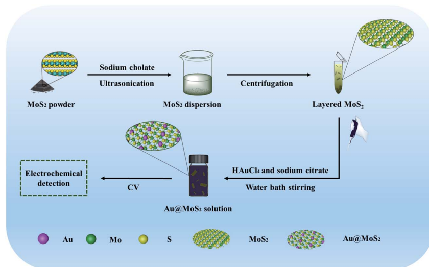
Scheme 1 The manufacturing process of MoS 2 nanosheets and Au@MoS 2 nanosheets and detection of the nanosheets.
