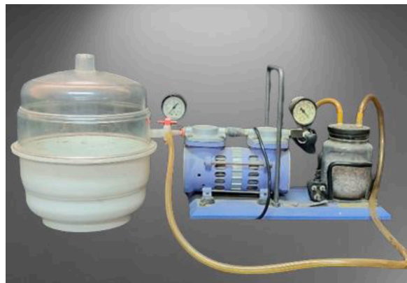
Fig. 2. Laboratory scale vacuum impregnation set-up.
