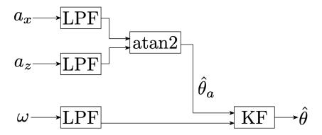
**Figure 7.** Flow chart outlining the process used to derive the pedal angle. After passing the analysisrelevant signals through second order Buttwerworth low-pass filter (LPF), we compute a rough estimate of the pedal angle based on accelerometer measurements  $\hat{\theta}_a$  and then fuse the gyroscope measurements  $\omega$  with  $\hat{\theta}_a$  using a KF to get a refined version of the estimate  $\hat{\theta}$ .
