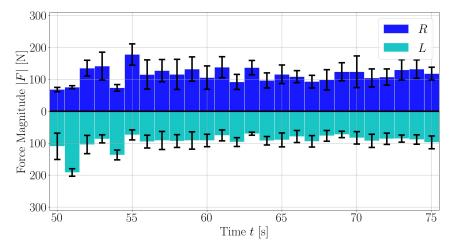
**Figure 10.** Average magnitude of the force exerted on pedal over time. Here, a section of a large assessment is shown. The averages are computed over 1 s bins. The bars' heights are the average force magnitude over the bin, and the error bars span plus and minus one standard deviation.
