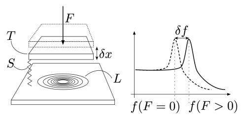
**Figure 3.** Load sensor working principle. By applying a force *F* to the target *T*, the spring *S* is gets displaced by  $\delta x$ . This change in target position causes the inductance *L* of the LC-tank to change, and thus causes a change in resonance frequency  $\delta f$ . By measuring the resonance frequency *f* of the LC-tank for various forces *F*, one can construct a mapping from *f* to *F* and thus estimate the forces based on the LC-tank's resonance frequency.
