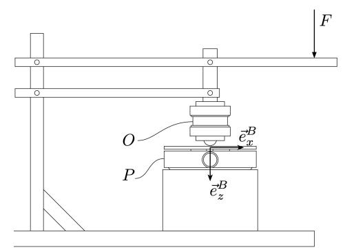
**Figure 6.** Schematic representation of the force-calibration setup. Depending on the mounting mode of the pedal *P*, the operator can apply forces *F* to *P* and collect, simultaneously, data coming from *P* and the reference sensor *O*. Three mounting modes are possible, enabling loading in  $F_x$ ,  $F_z$ , and  $M_x$ .
