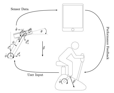
**Figure 2.** Graphical illustration of the pedal system. Users cycle on the ergometer, applying a force on the pedals. The pedals measure the load applied and transfers it to a tablet device for analysis. Audio or visual feedback is transmitted back to the user to provide feedback.
