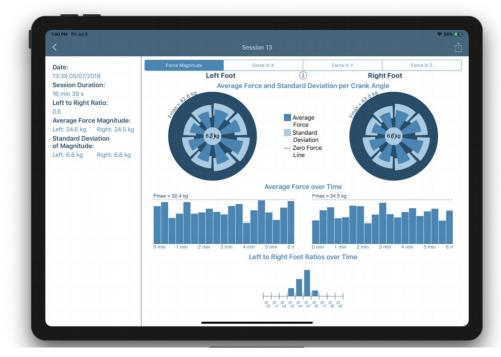
**Figure 11.** Pedalling forces breakdown. Post-session analysis showing breakdown of forces for different crank angles.
