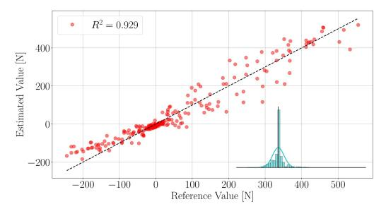
**Figure 8.** Force  $F_z$  model performance on test data set. The histogram represents the error  $e = F_z - \hat{F}_z$  distribution—the black vertical line is located at e = 0, the bins have size 6.15 N.
