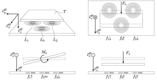
**Figure 4.** Working principle for 3D load detection using three coils. Here, a forward shear force  $F_x$  will cause a change in  $f_0$ , and the opposite change in  $f_1$  and  $f_2$ . Torque around the *x*-axis  $M_x$  would cause a change in  $f_1$  and the opposite change in  $f_2$ , with  $f_0$  remaining constant. Finally, a normal force  $F_z$  will cause all frequencies to change equally. With this, all load types can be differentiated.
