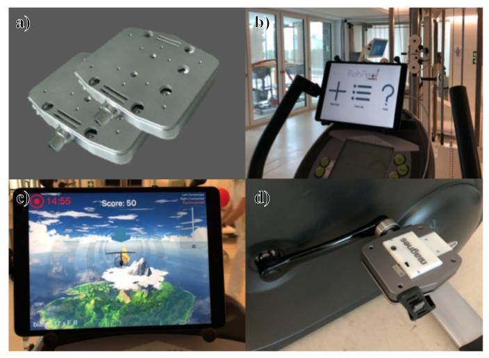
**Figure 1.** The developed ergometer-upgrade system. (**a**) 3D rendering of the sensor-equipped pedals; (**b**) The tablet mounted on an ergometer displaying the developed app's home view; (**c**) In-game view of a training session; (**d**) One of the pedals installed on the ergometer—here, the pedal is upside down.
