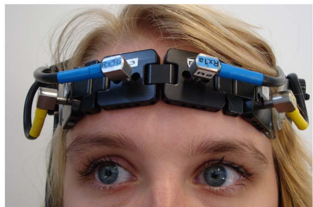
Figure 2. Positioning of the two pairs of fNIRS optodes. The subject of the photograph has given written informed consent (as outlined in the PLoS consent form) to publication of her image. doi:10.1371/journal.pone.0046210.g002
