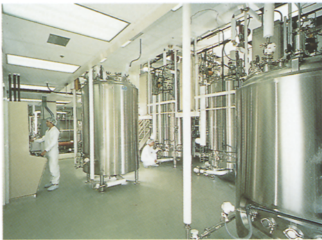
Fig. 4 Cell-culture area, with 2500-l bioreactors and harvest tanks
