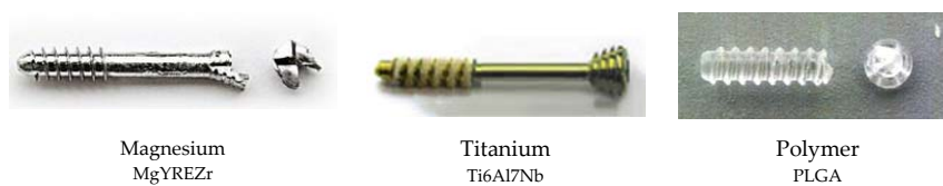
Figure 3. The screws after pull-out tests.
