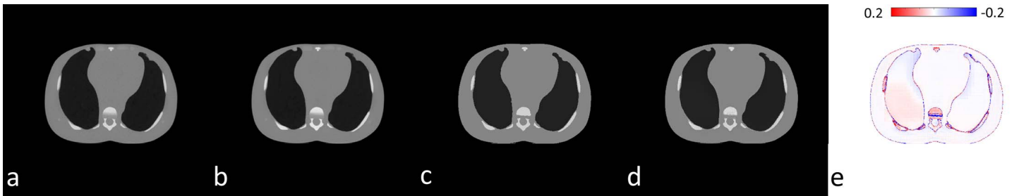
Figure 3. Axial views of phantom on (a) high-energy computed tomography images, (b) low-energy tomography images, and (c) its ground-truth relative stopping power (RSP) maps, and (d) RSP maps produced by the proposed method, respectively. (e) The difference maps of (d)–(c). The window level of RSP maps (c and d) is [0, 2].
