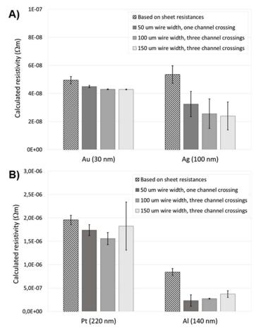
**Figure 4.** The resistivities of (**A**) Au and Ag metallizations and (**B**) Pt and Al metallizations calculated based on both measured sheet resistances of planar metal films and measured resistances of the metal wires (of different widths) travelling across the edges of Ormocomp microchannels one or three times.
