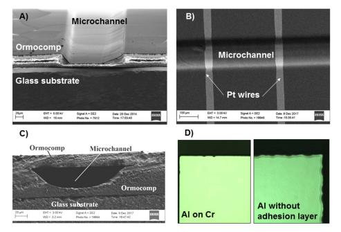
**Figure 3.** A scanning electron micrographs of (**A**) the cross-section of Ormocomp microchannel fabricated exploiting controlled overexposure ( $\geq 19 \text{ mJ/cm}^2$ ) and featuring tilted side walls, (**B**) Pt wires (50 µm wide, 220 nm thick) crossing an Ormocomp channel, and (**C**) the cross-section of a bonded Ormocomp microchannel. (**D**) Comparison of the etch profile of Al thin-film metal in AZ351B developer with and without adhesion layer (17 nm Cr).
