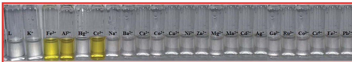
Fig. 3 The colour changes of L (10 \mu\text{M} ) upon addition of various metal ions (1 equiv.) in \text{CH}_3\text{CN-H}_2\text{O} (1 : 1, v/v) at room temperature.
