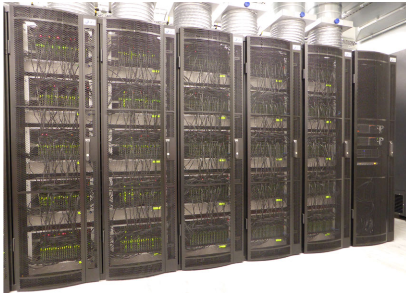
Figure 7. The 500 000-core SpiNNaker Human Brain Project platform. (Online version in colour.)
