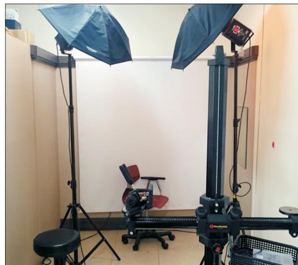
Fig. 5. Clinical photo room. The mirror on the wall was used to orient patient's natural head position by mirror-guided technique. The mirror is 150 cm far from the chair. The studio-stand on the bottom of the picture was set to be parallel to the gravity line, vertically, and perpendicular to the gravity line, horizontally by using a fluid level.
