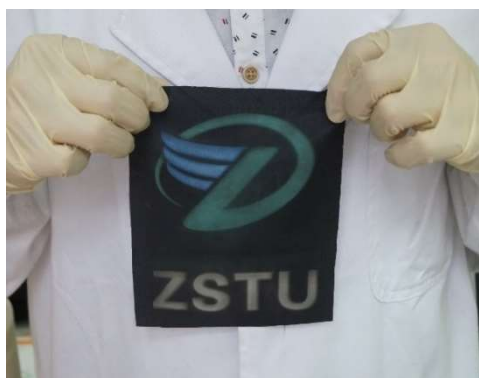
Figure 4. Structural color pattern of our university logo on polyester fabric.
