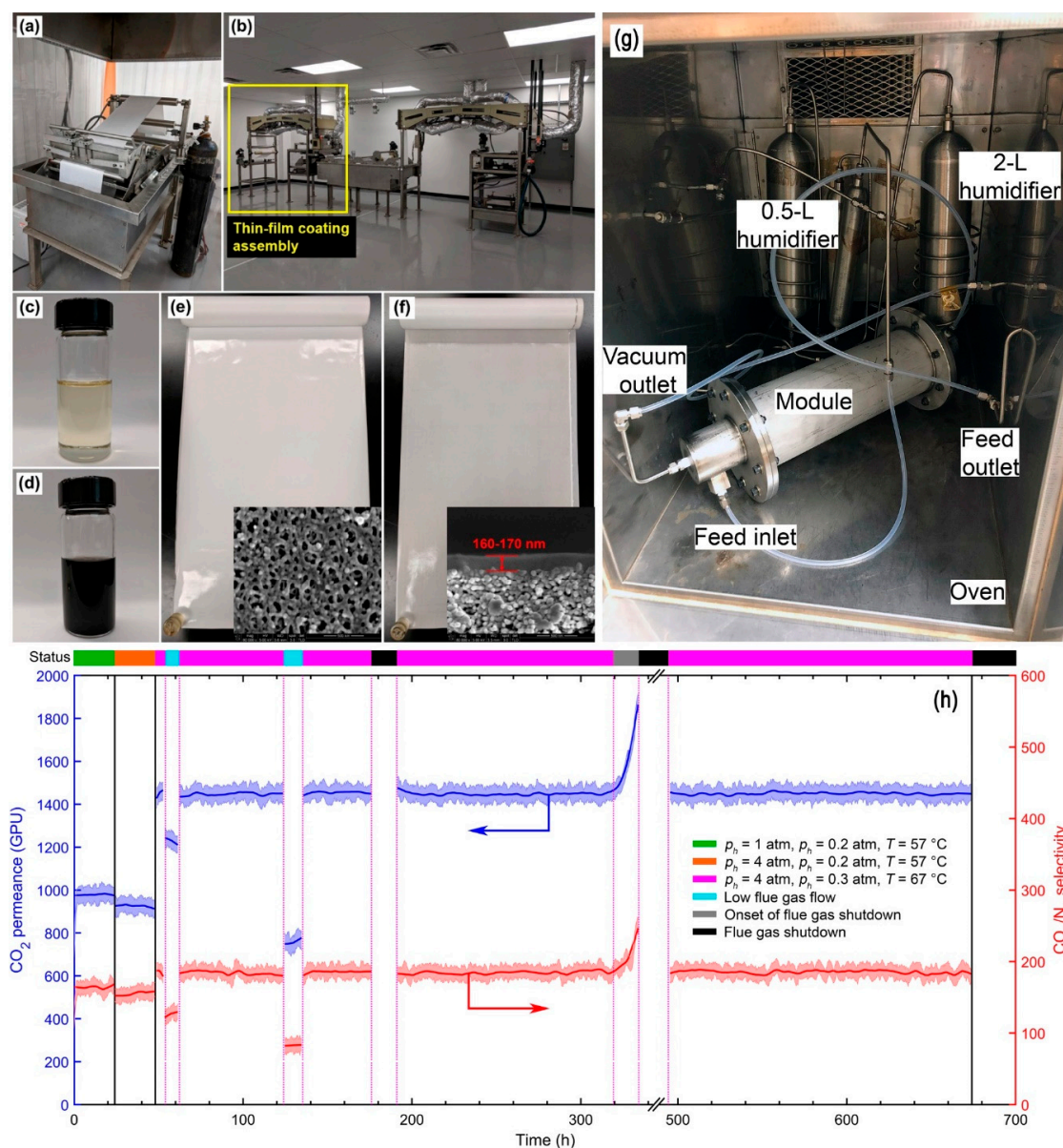
Figure 16. (a) Polymer support casting machine; (b) Thin-film coating machine; (c) PES casting solution for support fabrication; (d) Amine-containing coating solution; (e) 14''-wide scale-up PES substrate (insert: SEM of the PES surface morphology); (f) 14''-wide scale-up composite membrane (insert: cross-sectional SEM of the composite membrane's top layer); (g) Photo of OSU's 1.4-m 2 SW module at NCCC; (h) 500-h stability of the SW module. Reproduced with permission from [38,63]. Copyright Elsevier, 2019&2020.
