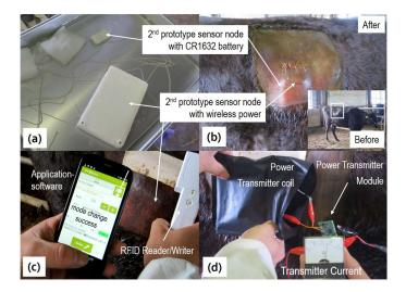
**Figure 6.** Photos of the sensor nodes ready for implant (**a**); the cow after implant (**b**); remote control test (**c**); and remote wireless charge test (**d**).
