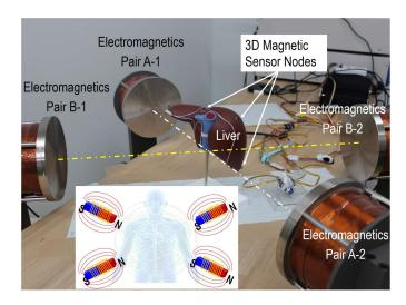
**Figure 9.** Photos and mechanism of the positioning system by using 3D magnetic sensors and artificial magnetic fields.
