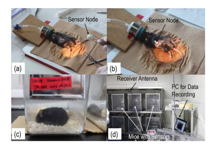
**Figure 3.** Photos of a mouse before (**a**), during (**b**), and after (**c**) implantation. Then, several mice were kept in cages to capture their body temperatures every few minutes (**d**).
