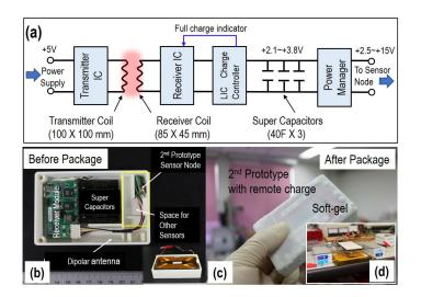
**Figure 2.** Schematic view of the wireless power transmission system, which includes a power transmitter module and power receiver module (**a**); photos of the second prototype sensor node with wireless power receiver module before (**b**) and after packaging (**c**); and photo of the evaluation system (**d**).
