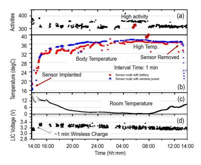
**Figure 7.** Evaluation results after implanting the second and third prototype sensor nodes into a wagyu (Japanese cow): calculated activities form the measured data of the accelerometer (**a**); measured body temperature (**b**); measured room temperature (**c**); and measured voltage of the LIC (**d**) for the duration of a day after implantation.
