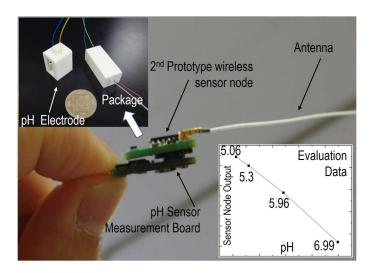
**Figure 8.** Photos of the developed fully solid wireless pH sensor before and after packaging. The inset shows the evaluation results collected by the wireless receiver.
