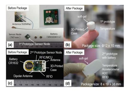
**Figure 1.** Photos of the first prototype sensor node and second prototype sensor node before (**a**,**c**) and after packaging (**b**,**d**) using the 3D-printed case, and then covering and filling with bio-compatible soft-gel.
