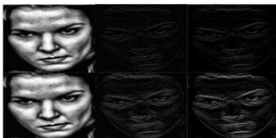
Figure 5. The illumination normalized expression samples of frequency domain transform based on WAVEDEC2 in RAF Compound. The upper row denotes illumination normalized expression samples of WAVEDEC2 transform based on sym1; the lower row denotes illumination normalized expression samples of WAVEDEC2 transform based on rbio3.1. Copyright reference: http://www.whdeng.cn/raf/model1.html#dataset .
