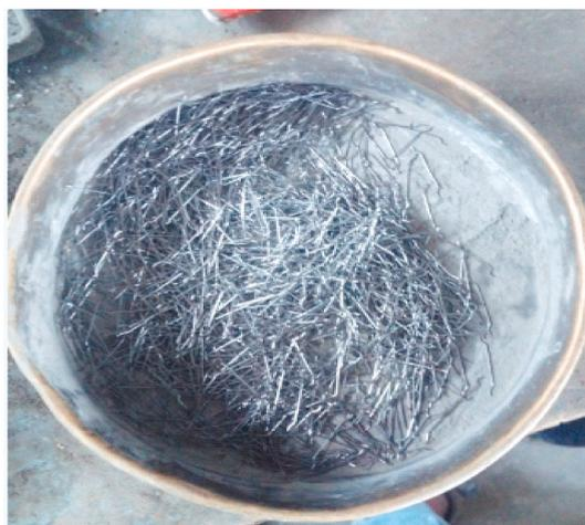
**Fig. 1.** Steel fibre.
