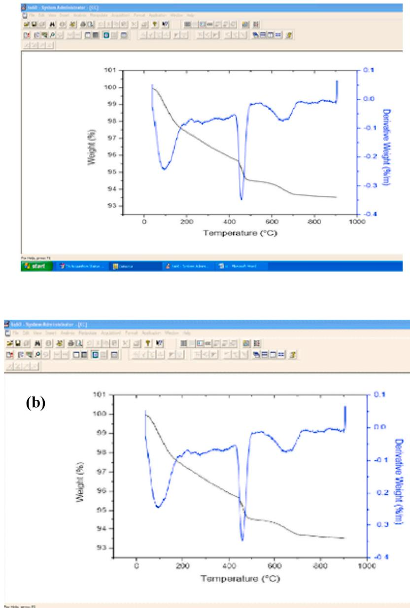
Fig. 13. TG analysis for (a) 7 and (b) 28 Days samples.
