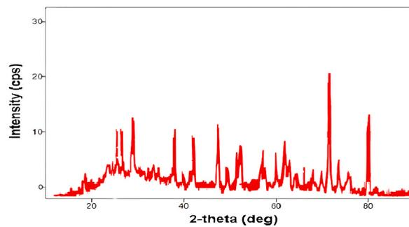
Fig. 12. XRD spectra for Carbon Black Sample.
