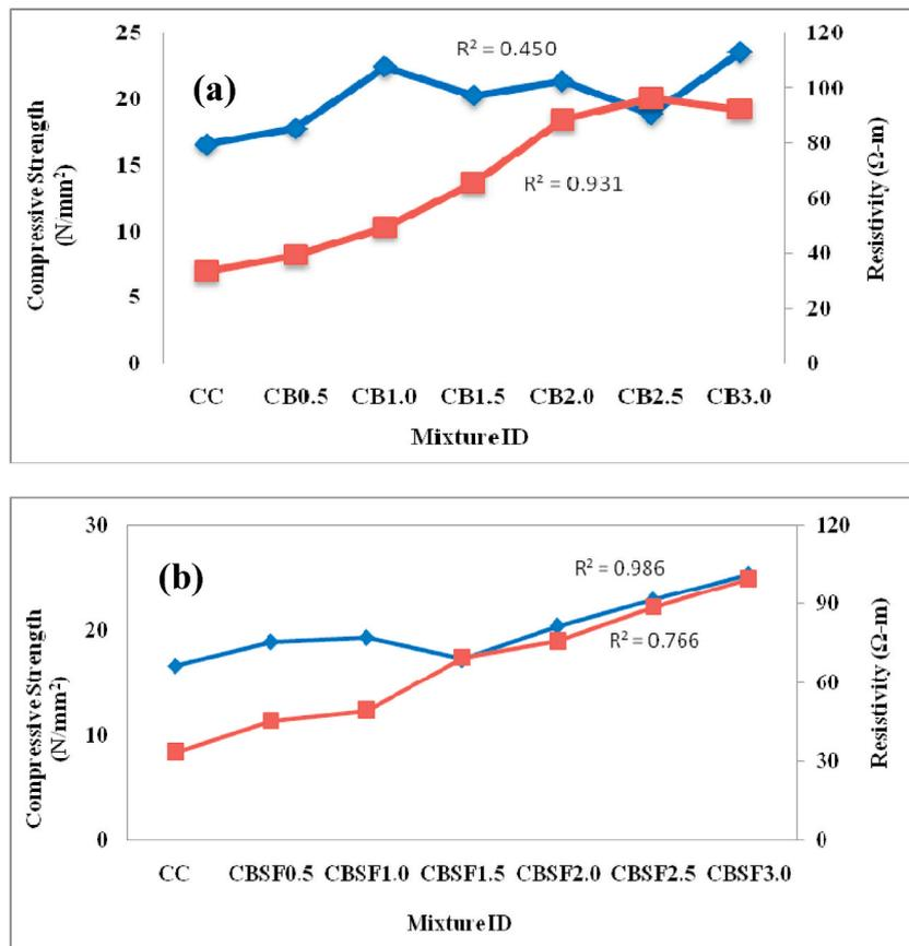
Fig. 5. Compressive Strength and Resistivity of concrete cube with (a) Carbon block and (b) Hybrid materials.
