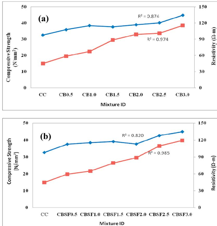
Fig. 9. Compressive Strength Vs Resistivity of concrete cube with (a) carbon black and (b) Hybrid materials.
