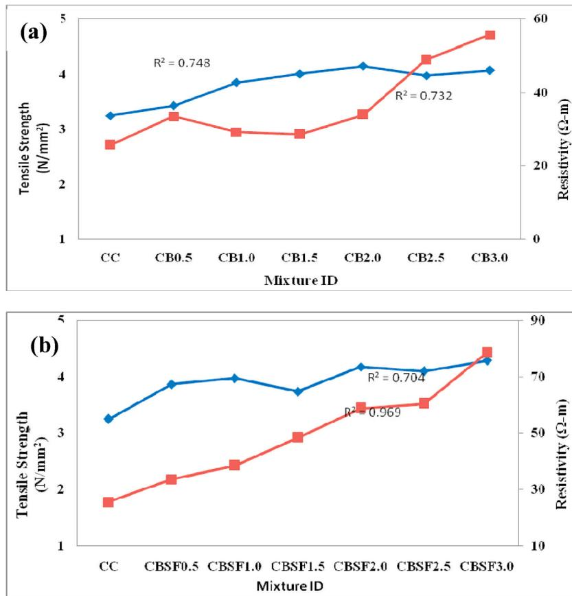
Fig. 10. Tensile Strength Vs Resistivity of concrete cylinder with (a) carbon black and (b) hybrid material.
