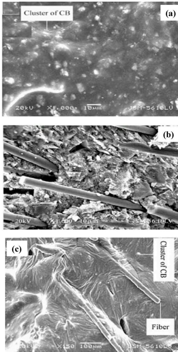
Fig. 11. Sem image of cement concrete with (a) carbon Black, (b) steel fibre and (c) hybrid carbon Black and steel fibre.
