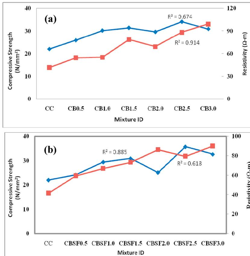
Fig. 7. Compressive Strength Vs Resistivity of concrete cube with (a) carbon black and (b) Hybrid materials.
