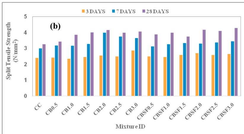
Fig. 4. (a) Compressive strength and (b) Split Tensile Strength of Concrete.
