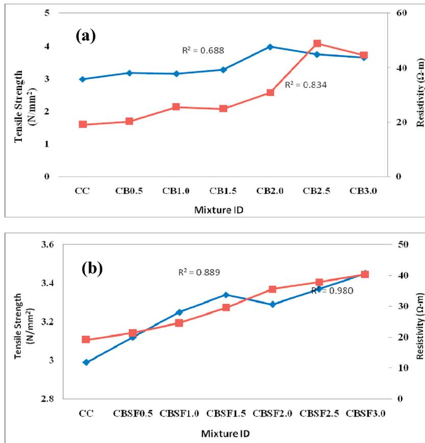
Fig. 8. Tensile Strength Vs Resistivity of concrete cylinder with (a) carbon black and (b) hybrid material.
