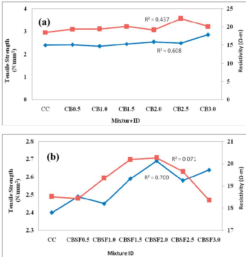
Fig. 6. Tensile Strength and Resistivity Vs of concrete cylinder with (a) carbon black and (b) hybrid material.
