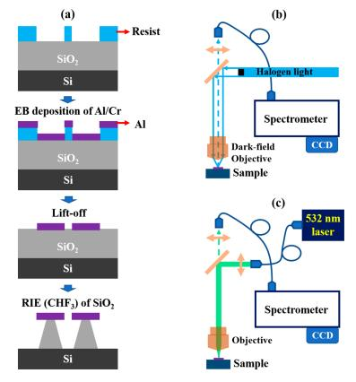
**Figure 1.** (**a**) Schematic illustration of the fabrication process. Optical microscopy setup of (**b**) dark-field measurement and (**c**) Raman measurement.
