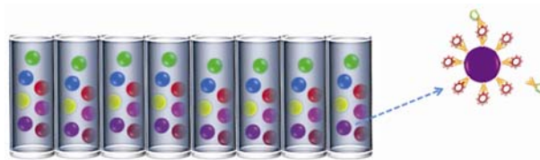
Figure 3 Scheme of suspension array. In each well, there are different microparticles and different immunoassay occurs on different microparticles instead of on different positions of a planar carrier.
