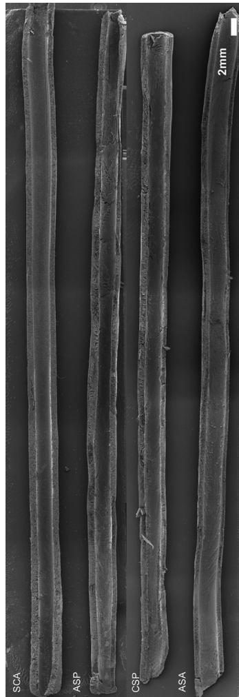
Fig. 1. Longitudinal sections of SCA, ASP, CSP, and ASA tubes.
