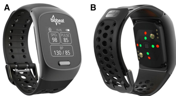
Figure 1. The Biobeat BB-613WP device. This PPG-based wearable provides non-invasive, cuffless, wireless and repeated measurement of blood pressure, heart rate, saturation, respiratory rate, stroke volume, cardiac output, cardiac index, systemic vascular resistance, pulse pressure, heart rate variability, mean arterial pressure, skin temperature, sweat, movement, and calories. Data is transmitted in real-time to a user App and to a medical management system. (A) The face side. (B) The back side with integrated sensors.
