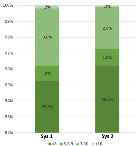
Figure 2. Percentage of measurements with a delta of less than 5, 5–7, 7–10 or above 10 mmHg between the reference device and the BB-613WP systolic measurements. Sys1 first systolic measurement. Sys2 second systolic measurement.
