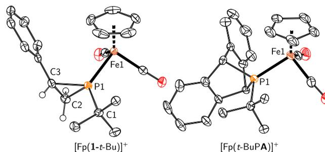
Figure 1. Molecular structures of [Fp(**1-t-Bu**)]-[BF<sub>4</sub>] and [Fp(*t*-BuPA)][BF<sub>4</sub>] with thermal ellipsoids set at the 50% probability level. Selected hydrogen atoms and the tetrafluoroborate anions have been omitted for clarity. Selected bond distances and angles (Å, °) [Fp(**1-t-Bu**)]-[BF<sub>4</sub>]: P1–Fe1:2.2283(6); P1–C2:1.811(2); P1–C3:1.846(2); C2–C3:1.524(3). [Fp(*t*-BuPA)][BF<sub>4</sub>]: Fe1–P1:2.258(2).
