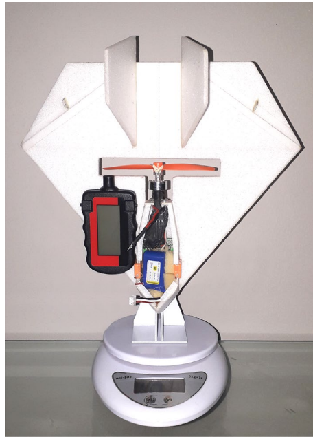
Figure 24. Digital scale with high-precision and digital spin counter HCAP0400 used for static thrust determination.
