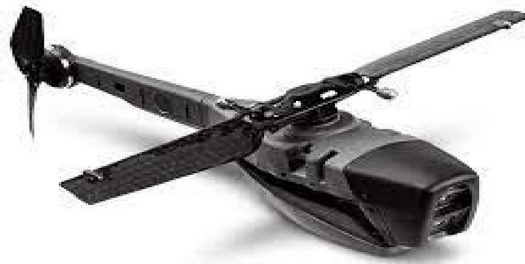
Figure 4. The Black Hornet micro UAV, it partially fits the needs of our project, but flight distance. Black Hornet measure is 0.168 m, overall, and its weight is 0.033 kg.
