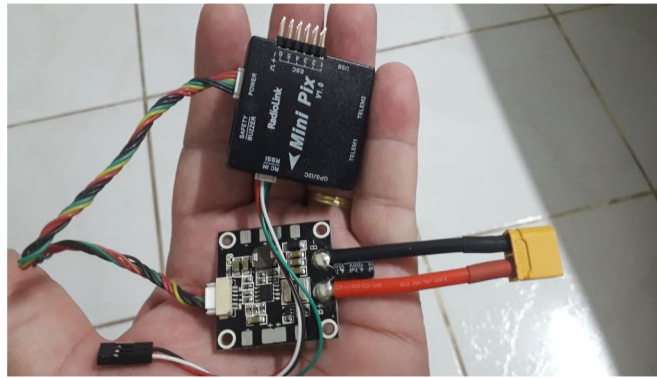
Figure 20. Autopilot embarked in the prototype.
