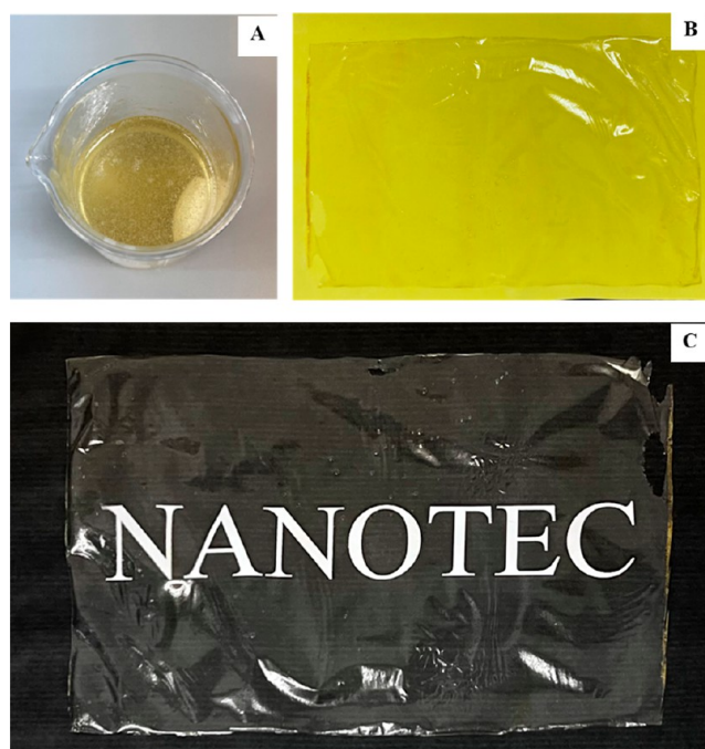
Figure 10. Bionanocomposite film by doctor blade process using PVA as a processing aid. (A) Solution of D-chitosan in bioacid with PVA, (B) film casted by doctor blade on brown paper, and (C) film on black paper printed with white letter "NANOTEC".
