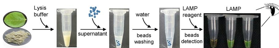
**Figure 1.** Schematic show of PAMMPs@DNA-LAMP. The DNA is purified by being rapidly captured on PAMMPs, and PAMMPs@DNA is directly detected by LAMP. The LAMP result is visually detected by directly adding SYBR Green I (visual PAMMPs@DNA-LAMP).
