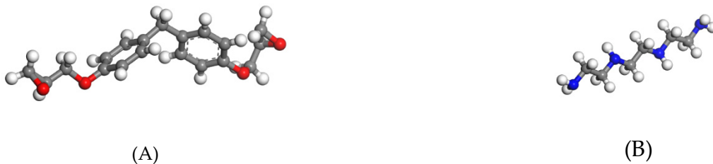
Figure 1. Epoxy resin monomer and curing agent: (A) DGEBF; and (B) TETA.
