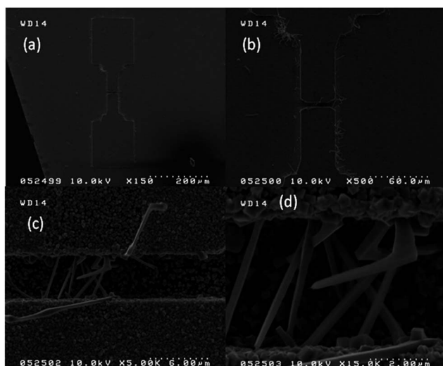
Fig. 3 (a) Low magnification SEM image of Si electrodes on SOI wafer for first ITZO device. (b) ITZO nanowires are seen both on Si electrode sides and gap between Si electrodes. (c) High magnification SEM image of a gap between Si electrodes on a SOI wafer. (d) High magnification SEM images of bridged ITZO nanowires that grown between Si electrodes. As seen from the SEM images, only 6 ribbon shaped nanowire are connected to two the Si electrodes.
