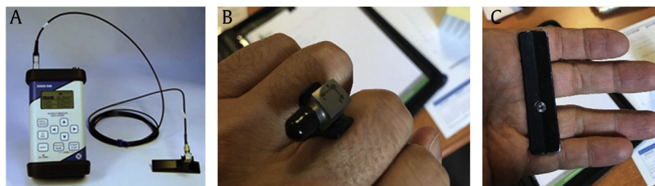
Fig. 3. The analyzer used to collect the vibrations (A) made of an accelerometer (B) and an handle equipment (C) to hold the accelerometer.
