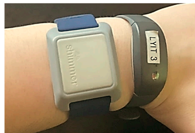
Figure 1. Verisense (left) and Actiwatch 2 (right) wrist-worn devices as worn by a participant.
