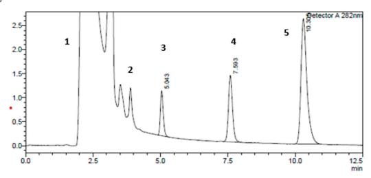
**Figure 3.** Typical HPLC chromatogram of CYP2E1 components with standard rat microsomal medium (40 min incubation of chlorzoxazone) at 282 nm wavelength detection with a 200-μM chlorzoxazone concentration. The peaks marked are: (1) the nicotinamide adenine dinucleotide phosphate hydrogen (NADPH)-regenerating system, (2) salicylic acid, (3) 6-hydroxychlorzoxazone, (4) phenacetin, and (5) chlorzoxazone, respectively.
