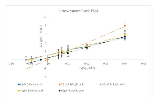
**Figure 4.** Representative Lineweaver–Burk plot for the inhibition of CYP2E1-catalysed chlorzoxazone 6-hydroxylation (chlorzoxazone (25–200  $\mu$ M)) with 0, 10, 25, 40, and 60  $\mu$ M salicylic acid. Each point represents the average of three determinations.
