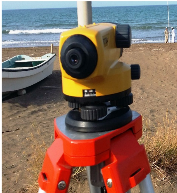
Figure 6. Leica Automatic Level used during the field measurements.
