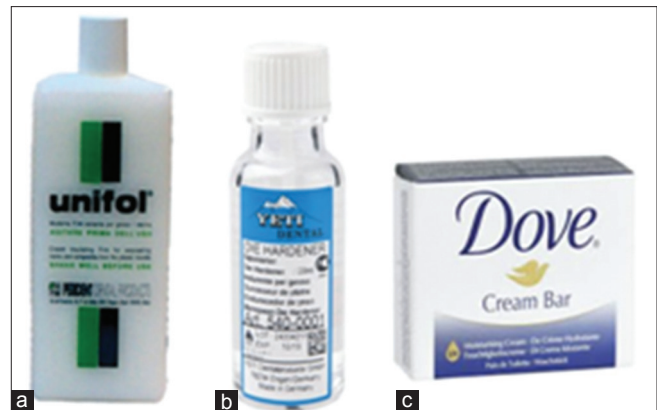
Figure 2: Separating media used: (a) Unifol, (b) die hardener, and (c) soap solution
