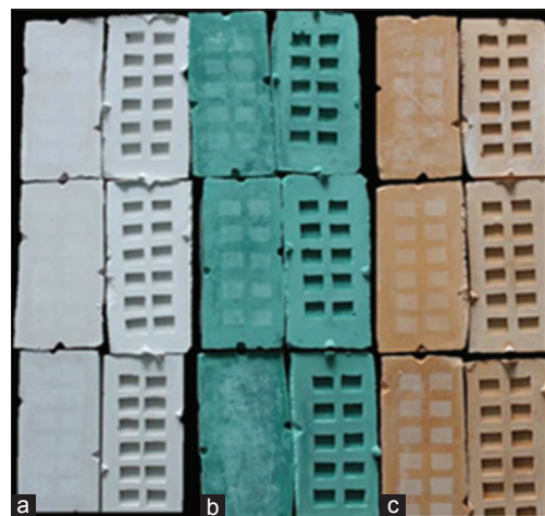
Figure 3: Molds fabricated using various materials: (a) Dental stone (white), (b) dental stone (green), and (c) die stone (orange)
