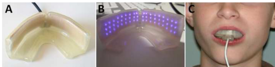
Fig. 2 OrthoPulse™ mouthpiece. Panel a displays a view of the back of the device. Panel b showcases the LED array when the device is switched on. Panel c provides a view of the device in situ
