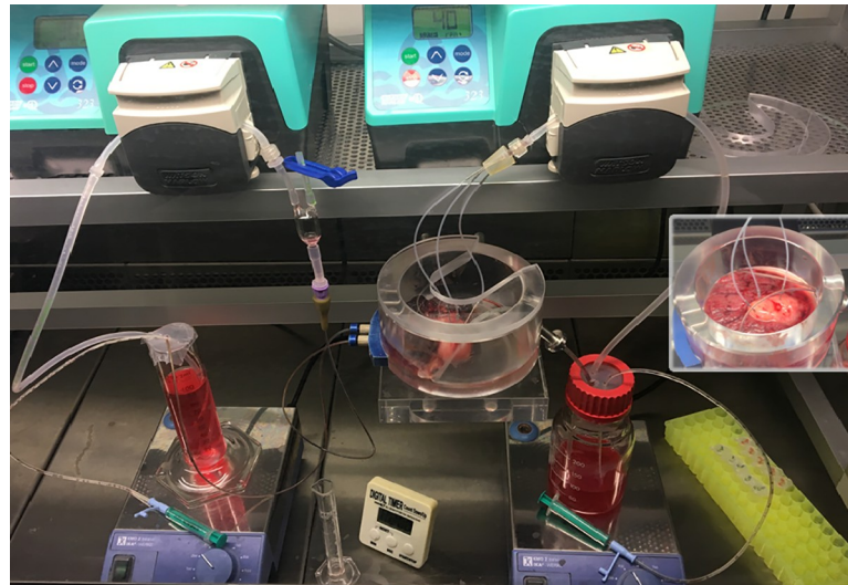
Fig 1. The placental perfusion system set-up. The full picture shows the perfusion set-up in the heated flowbench. At the left is the fetal reservoir and tubes with bubble-trap recirculating perfusion medium. In the middle is the placental lobule in the perfusion chamber. At the right is the maternal reservoir and tubes, recirculating medium, with three maternal cannula and gravitational collection of the outflow. The small cutout picture at the right is a closer view of the lobule and the three maternal cannula, with the light colored cotyledon caused by absence of blood.
