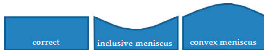
Figure 3. The issue of a convex and concave meniscus, casting in silicone.
