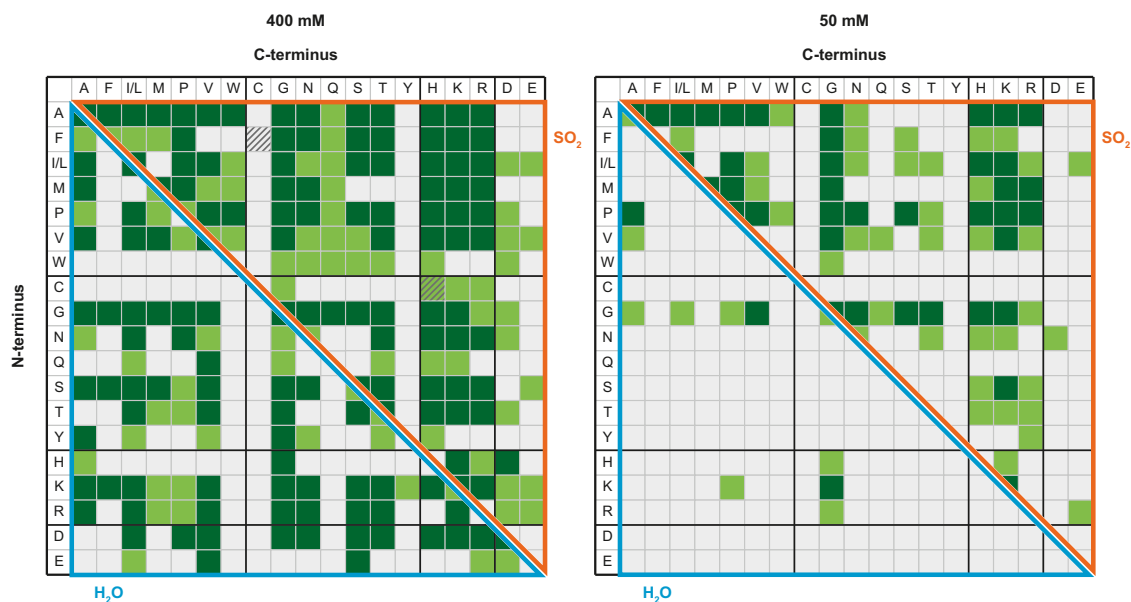
Fig. 5 Product spectrum of the complete amino acid mixture. Comparison of the detected dipeptides of copper-catalyzed peptide condensation in SO 2 and water after 21 d starting from 400 mM or 50 mM of the complete set of proteinogenic amino acids (dark green = confirmed by MS/MS, light green = traces, white = not detected, hatched = cystine-peptide traces). The CuCl 2 concentration in SO 2 was 5 mol% in both experiments. Amino acids are represented corresponding to the one-letter code.
