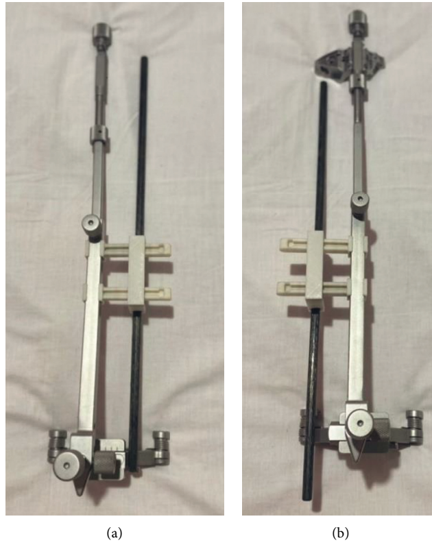
FIGURE 10: The tool can be fixed for both right and left sides. (a) Right leg. (b) Left leg.
