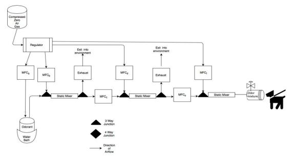
**Figure 1.** Schematic of the air-dilution olfactometer. Air flow path is shown from left to right and dog is shown evaluating the odor port. Briefly, compressed zero air is used to collect odorant from a sealed glass odorant jar in a water bath. The vapor stream is then systematically diluted using mass air flow controllers and turbulent static mixers. The odor line is then delivered to the odor port.
