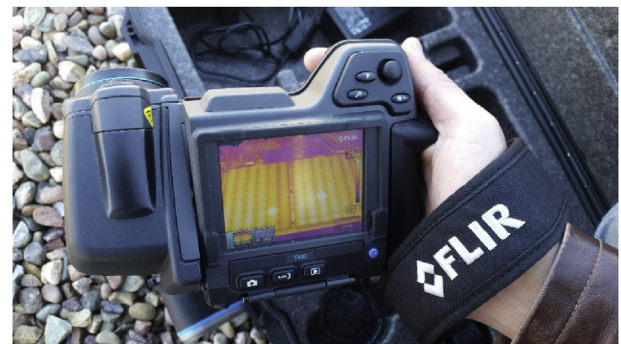
Figure 3. Flir T440 thermal camera used in this study.
