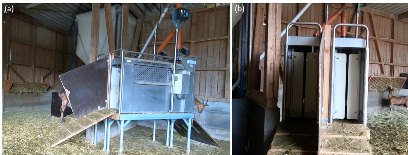
Figure 2. Photographs of the new optimized automatic feeding system. (a) The station in side view. (b) The divided entrance with the ramp.
