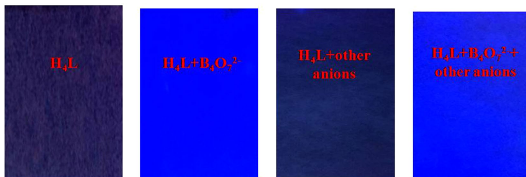
Figure 5. Photographs of the colorimetric test kit with H_4L for detecting B_4O_7^{2-} under irradiation at 365 nm.
