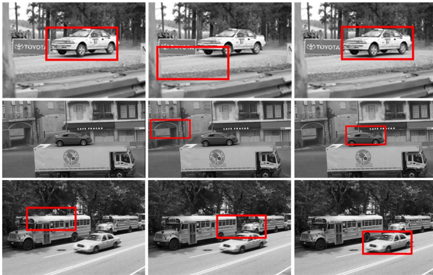
Figure 8. The car detection results with background clutter on the Pascal VOC 2008. For each row, the left image is the result of template matching; the middle image is the results of local Gist based template matching; and the right image is the results of the proposed method. doi:10.1371/journal.pone.0098447.g008
